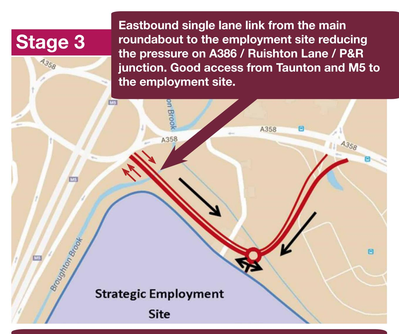
A single lane link in the eastbound direction could be delivered by providing the infrastructure for this link only however in the longer term it is likely that the link will need to be a dual carriageway when it connects to an improved A358 (Highways England scheme). Providing the base infrastructure at this stage would be more cost effective and limit disruption in the longer term.
