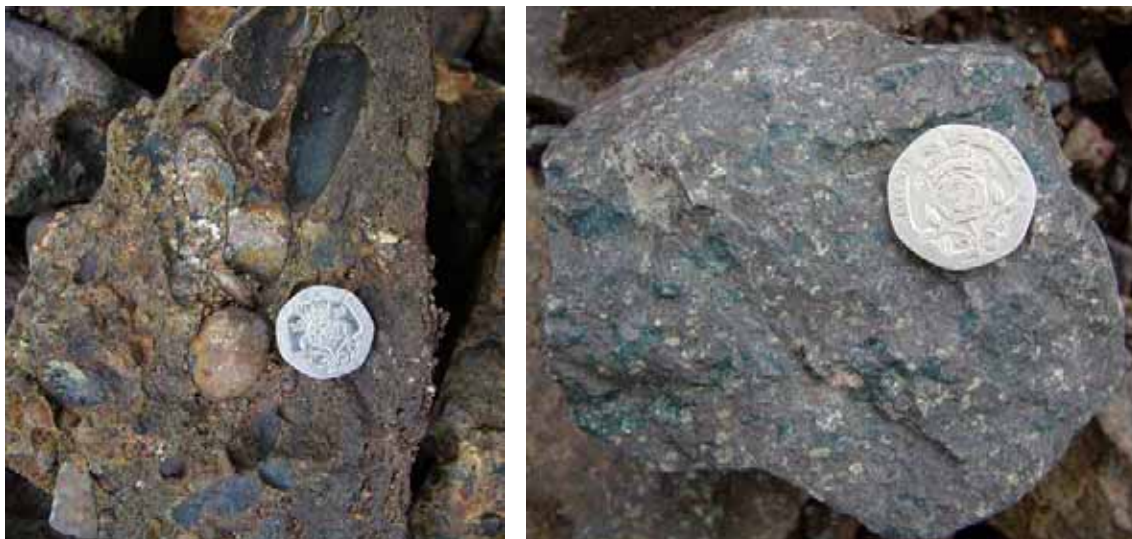
Photo PO 6 Moons Hill Quarry Typical examples of weathered agglomerate and fresh tuff Photo refs MH04j and MH08j Hand specimens
